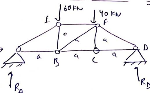
$$\begin{aligned} \sum F_x &= 0 \\ R_A &= 0 \\ \sum F_y &= 0 \\ R_A + R_D - 60 - 40 &= 0 \\ R_A + R_D &= 100 \end{aligned}$$
