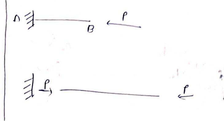
NOTE  $\Rightarrow$  All the tensile forces are going away from joint.
